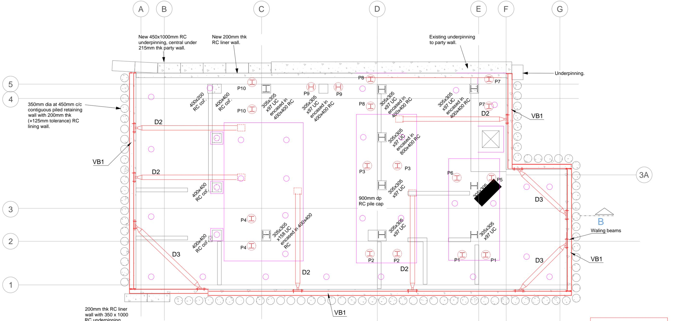
200mm thk RC liner wall with 350 x 1000 RC underpinning
